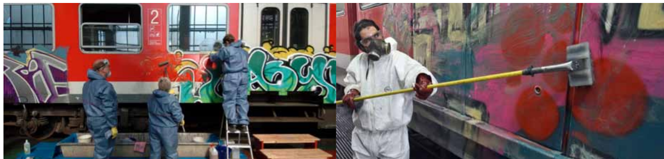
Fig.6 - Most graffiti on public transport is removed by hand using chemical solvents. Germany. 2013. Photos by Die Welt.
