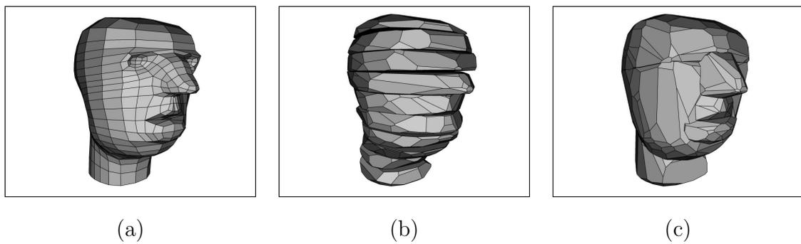
Fig. 15. Dual convex-hull results with subdivision: (a) Input mesh. (b) Dual convex-hull with uniform uniform clustering along y axis. (c) dual convex-hull with manual subdivision.
