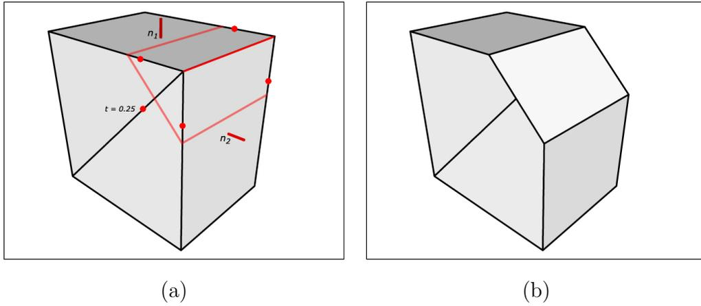
Fig. 7. Planar edge truncation:(a) The position and the normal of the slicing plane is computed based on the selected edge. (b) The selected edge is truncated by the computed slicing plan.
