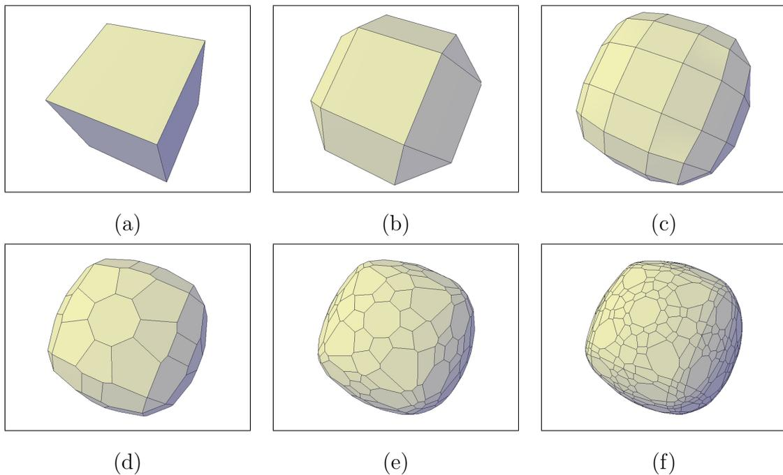
Fig. 22. Step by step creation of a pattern: (a-c) Two iterations of Doo-Sabin subdivisions are applied to a cube. (d) Planar face truncation is applied with 0.75 offset value to all faces. (e-f) Planar vertex truncation is applied for 2 iterations with 0.75 offset value.
