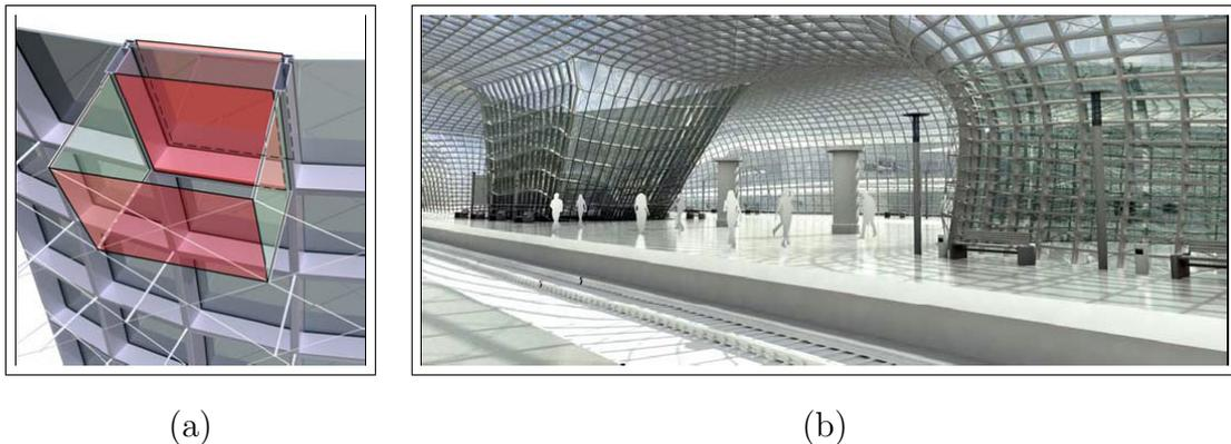
Fig. 4. (a) Offsetting a conical mesh results in the same connectivity. (b) A possible glass structure which is a conical mesh
