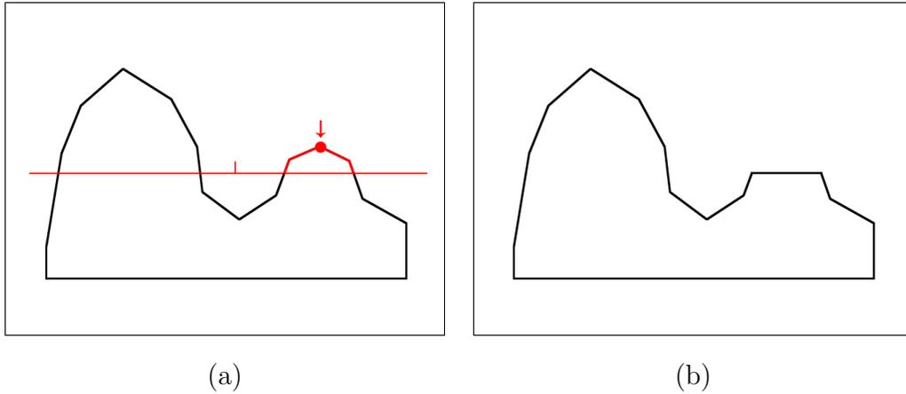
Fig. 6. (a) Local cutting starts traversing the mesh from a given element and continues until the slicing plane is hit.
