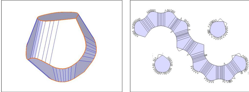
Fig. 18. A dodecahedron constructed from 3 pieces. This D-form is particularly interesting since the middle piece turns and touches itself.
