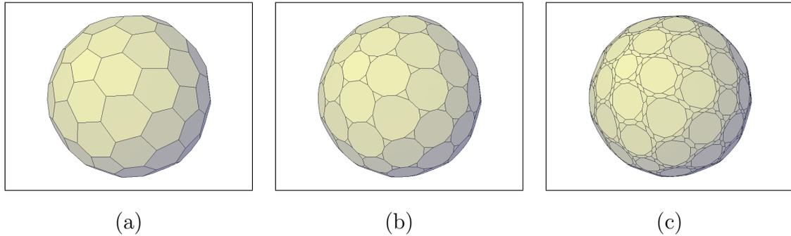
Fig. 12. (a) A honeycomb subdivision and planar face truncation applied to a soccer ball. (b) Planar vertex truncation applied to the shape successively. (c) Planar edge truncation is applied to the shape
