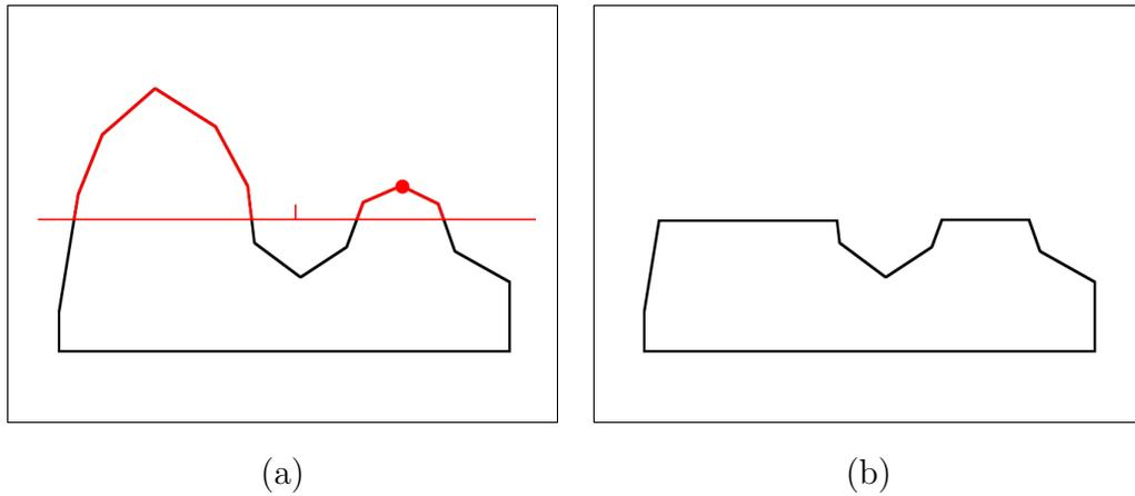
Fig. 5. (a) The default cutting algorithm traverses all the edges and marks all edges above the slicing plane for deletion.
