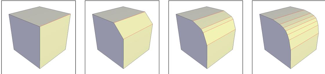
Fig. 10. The edge of a cube is smoothed out by truncating parallel edges.
