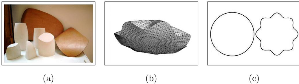
Fig. 3. (a) D-forms examples created by Tony Wills [22]. (b) A wireframe of a D-form. (c) A circle and a rippled shape with equal perimeters to create the D-form in (b).
