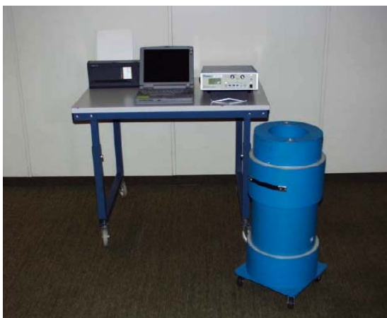
Figure 1.2. High Level Neutron Coincidence Counter.
