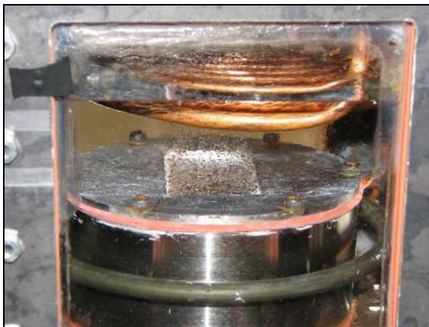
Fig. 39. Digital photograph showing pool boiling on a bare test surface under 20 °C sub-cooling condition very close to CHF
