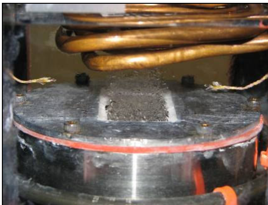
Fig. 40. Digital photograph showing pool boiling on the "336 nm" test surface under 20 °C sub-cooling condition very close to CHF
