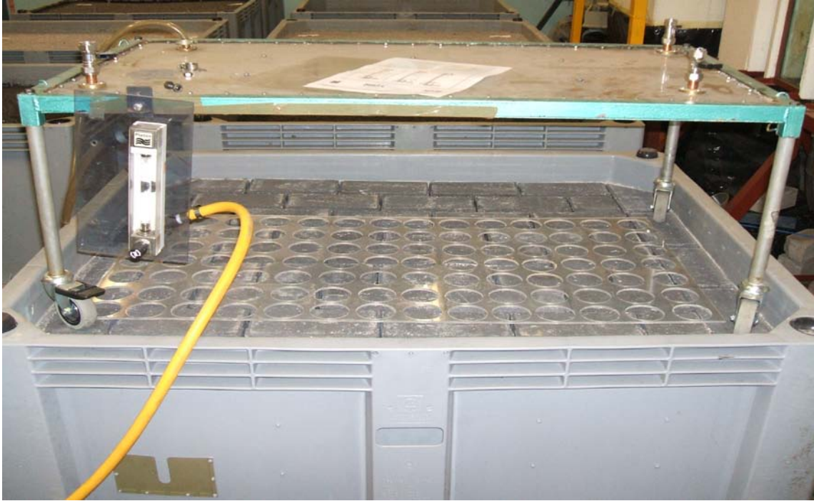
Figure 3.3 Showing Rainfall Simulator on a Test Model and Perspex Quadrat
