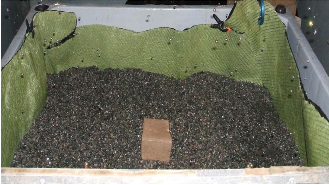
Figure 7.11 2 nd Test: Sub-Base, Geotextile and Bedding Layers
