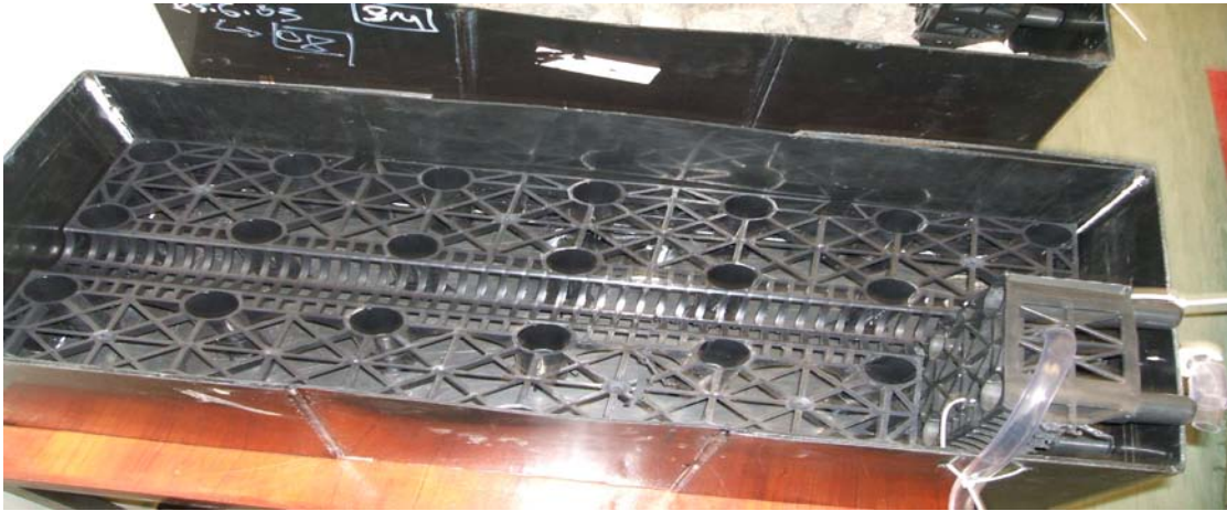
Figure 4.2 Experimental Rig Showing Permavoid Sub-Base
