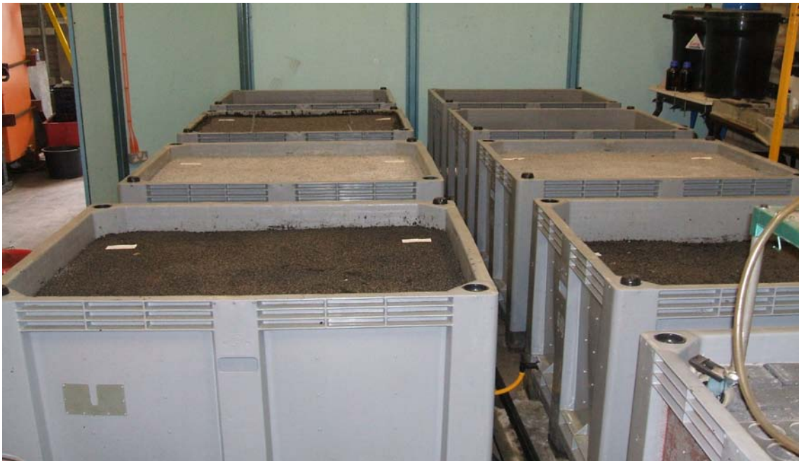
Figure 3.2 Test Models Arranged in the Laboratory in Coventry University-Plastic Barrels to the Rear Contain the Laboratory's Effluent Treatment System for Treatment of Excess Effluent
