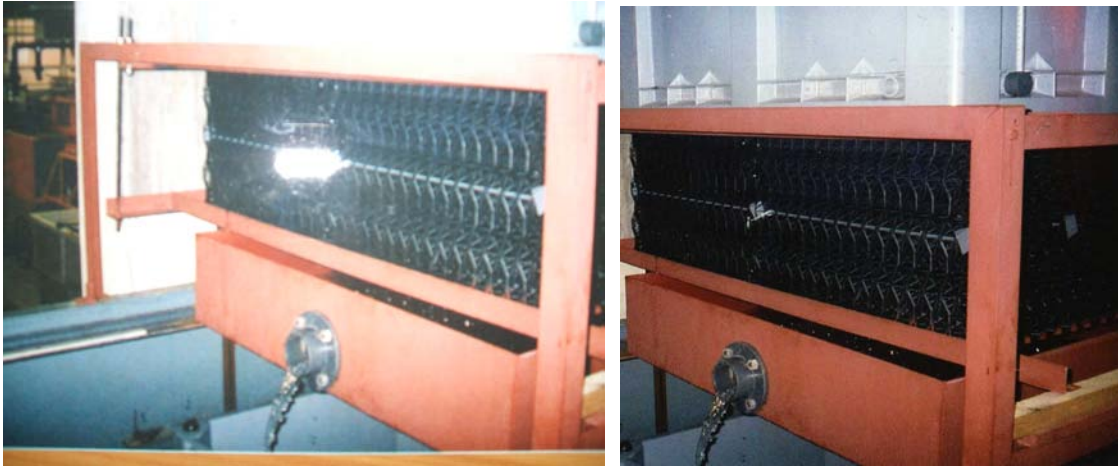
Figure 7.7 Water Rushing Out of Outlet Made in Metal Tray Mounted on Test Rig During Measurement of Intensity of Simulated Rainfall
