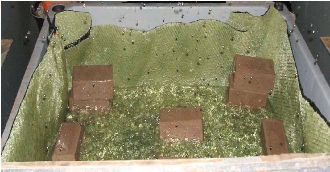
Figure 7.10 1 st Test: Sub-Base Layer and Geotextile
