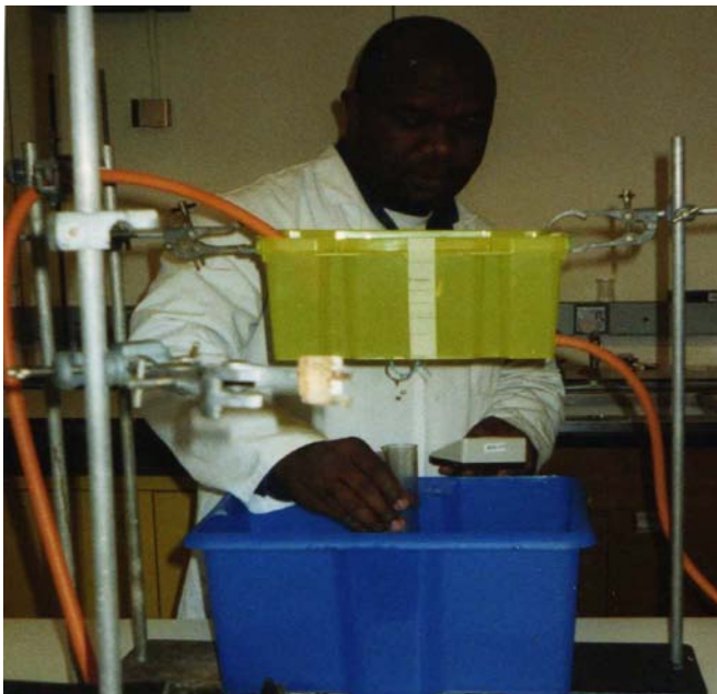
Figure 7.2 Small scale test measurement of rainfall intensity
