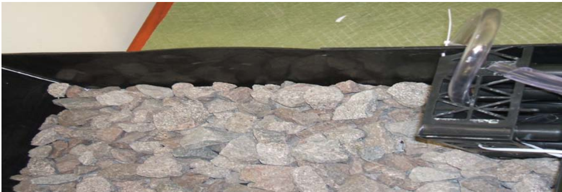
Figure 4.3 Experimental Rig Showing Stone Sub-Base
