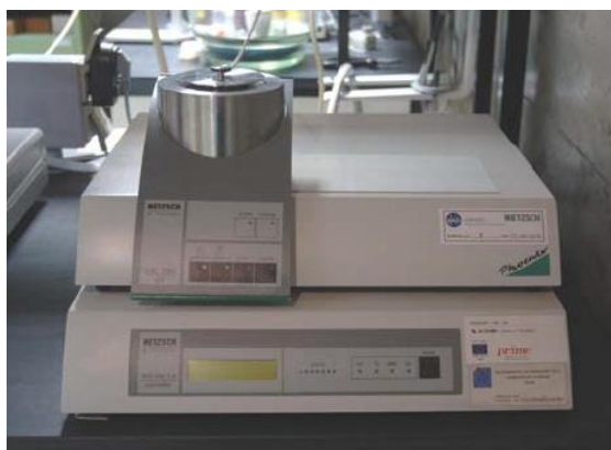
Figure 4-2 DSC (top) and temperature control unit (bottom)
