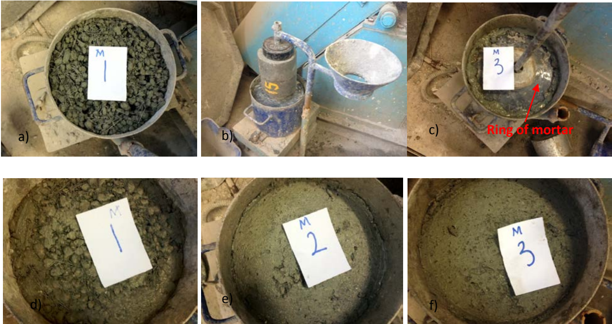
Figure 5.3: Representative mixtures: (a) M1 in the Vebe cylinder (b) 22.7 kg surcharge mass mounted on test specimen (c) Fully consolidate test specimen with a ring of mortar around the disk (d, e, f) Top finished surface of Mix 1, Mix 2 and Mix 3 after consolidation
