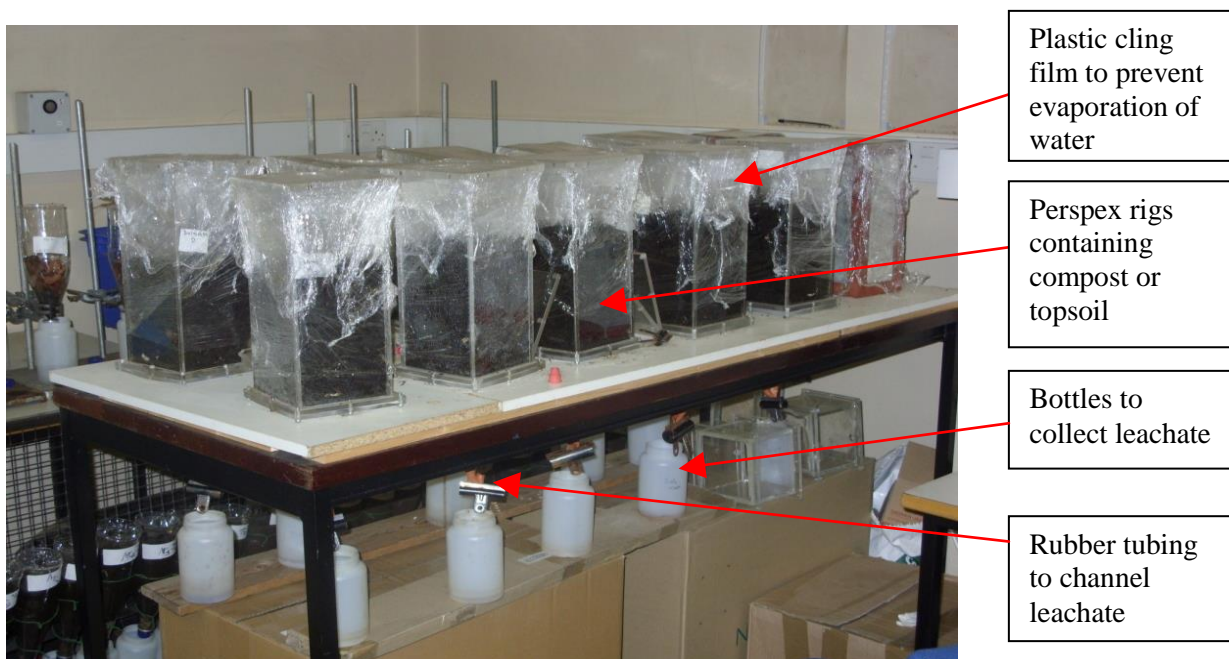
Figure 3.1: The experimental set up for determining water holding capacity
