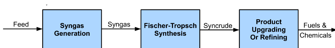
Figure 1.2: Flow diagram highlighting the main stages of FTS.
