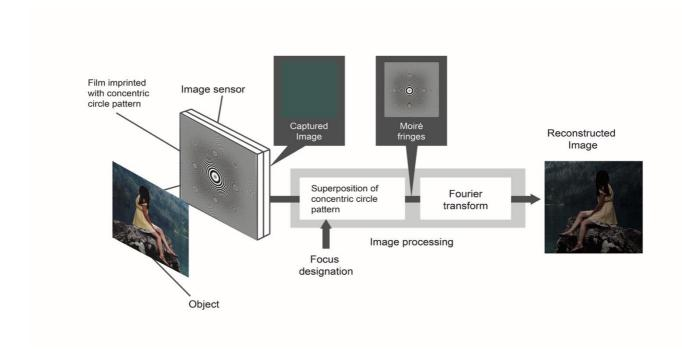
Fig. 12: Hitachi's lens-less camera operation
