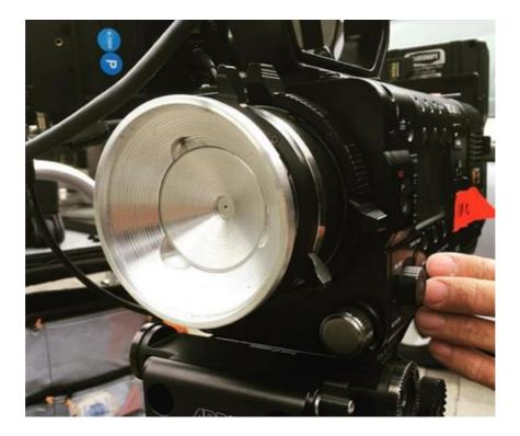
Fig.9: Joseffer's 75mm pinhole aperture camera attachment.
