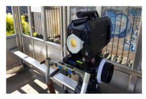
4K Black Magic cinematography camera with self-produced multiple pinhole disc (0.35mm) 800 ISO (noon sun, May 2017).
