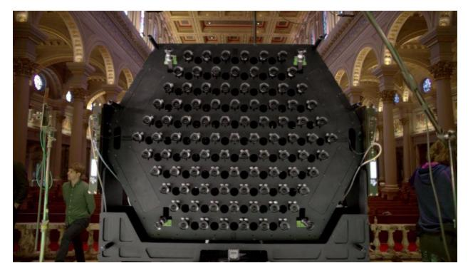
Fig.15: Lytro Immerge Camera with its multi-lens array generating light data which involves a huge amount of post-capture calculation. (Image: Lytro, 2016).
