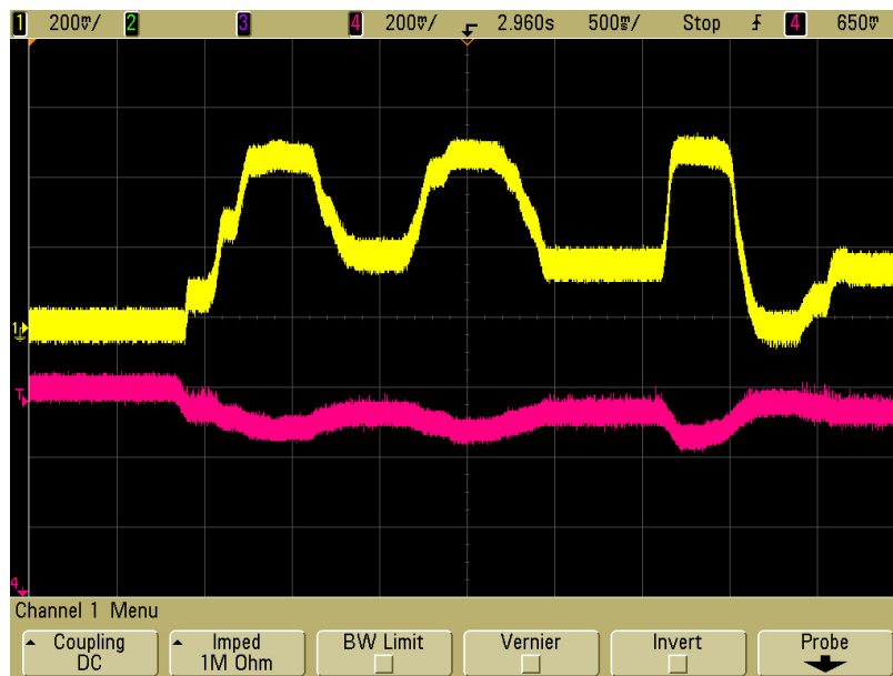
Fig. V.2. Bulk Node Voltage Modulation with VDD
