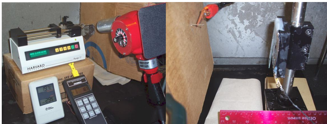
Figure 6. Convectively Heated Cellulose Setup, "Setup C"
