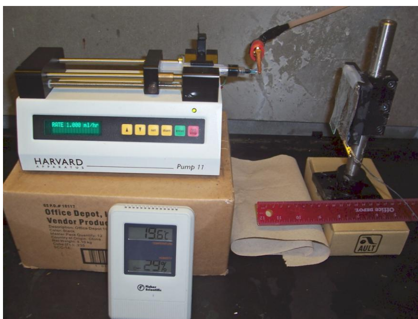
Figure 7. Cellulose with SWNT Simple Electrospinning Setup
