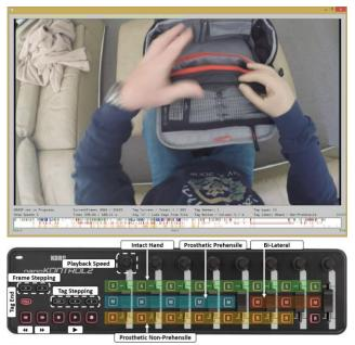
Figure 5: A screenshot from the custom video player software (top). Logged tags are shown in the playback progress bar. A hardware midi interface (below) is used to precisely control video playback and tagging.
