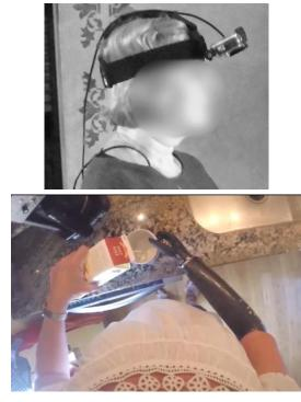
Figure 1: (Top) A head-mounted camera recorded the arms and hands of upper limb amputees as they performed self-selected tasks in their own homes. (Bottom) An example ego-centric frame from the camera.
