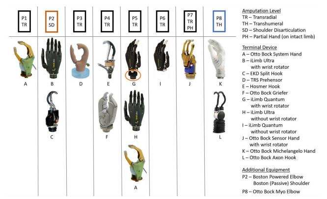
Figure 3: Terminal devices used by the participants during the study. All participants used their prosthetics devices every day, and had done so with their current prosthesis/prostheses for at least 6 months. P2 and P8 are highlight as non-transradial amputees.
