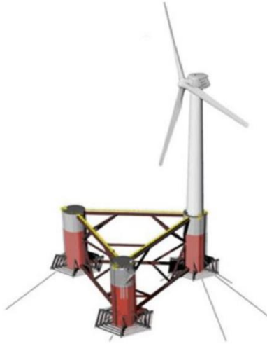
Fig. 1 The WindFloat platform [33].
