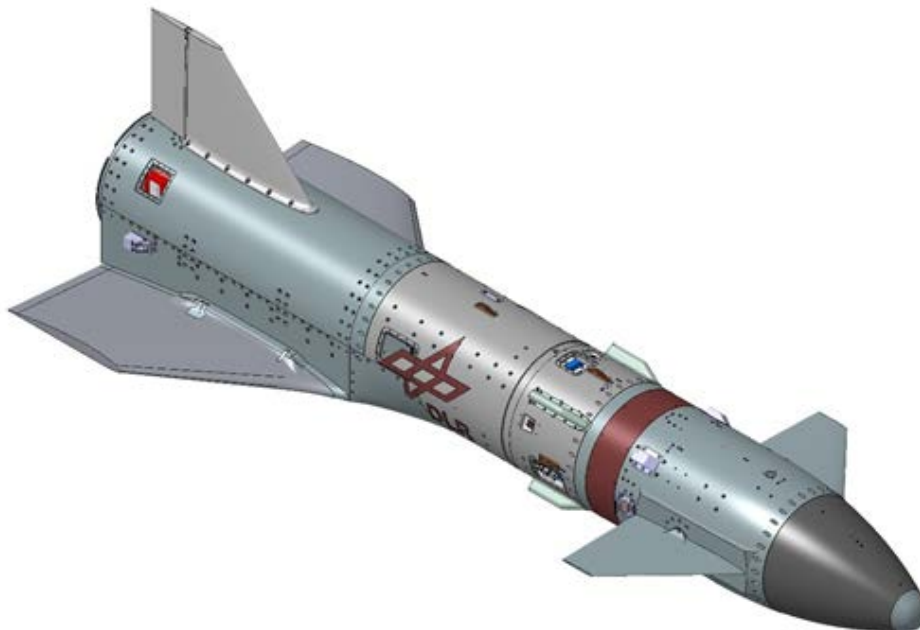
Figure 2: CAD Model of the ReFEX Re-Entry Segment
