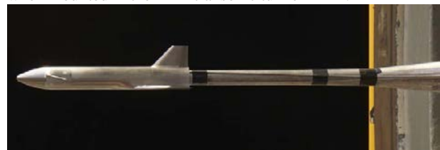
Figure 7: Model of ReFEX in DLR's windtunnel TMK in Cologne
