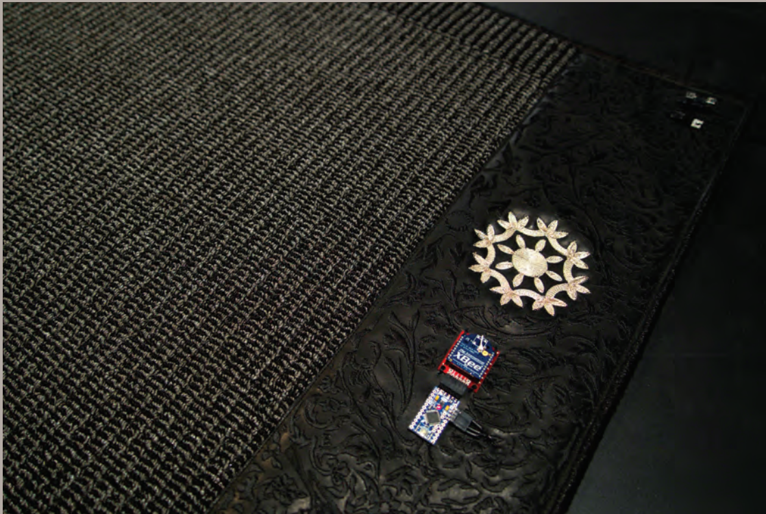
Detail of Sensing Carpet showing embroidery on leather with laid antenna, Arduino microcontroller and X-Bee transceiver.
