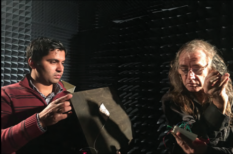
Tahseen Mustafa and Martin Peach test the efficiency of textile antennas in the anechoic chamber.
