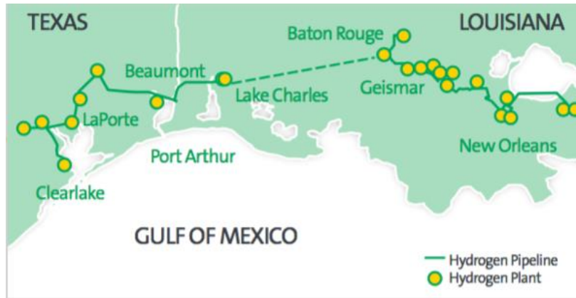
Figure 22.2 The map above shows Air Products' extensive Gulf Coast Hydrogen pipeline system. It is the world's largest hydrogen pipeline and reaches over 600 miles, stretching from Houston to New Orleans (Air Products, 2012).
