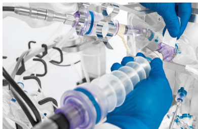
Figure 7. Bioreactor probe assembly.
