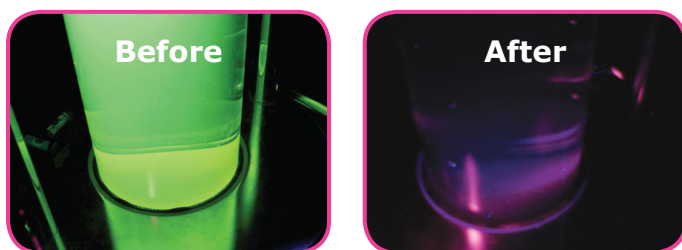
Figure 2. Before and after images of riboflavin presence (green) in a 100 mm QuikScale® column
