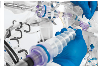
Figure 6. Bioreactor probe assembly.
