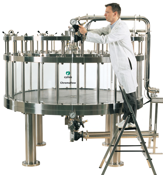
Fig 1. A Chromaflow column, 2000 mm i.d.
