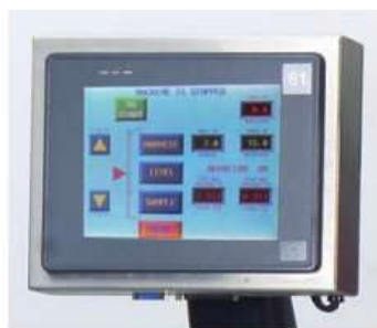
Fig 2. The touchscreen provides easy access to all control functions.
