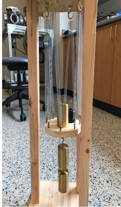
Figure 2.11: A test frame with 8 angled springs
