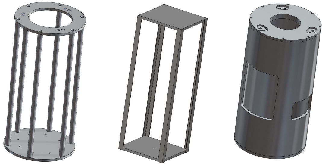
(a) Case 1: six circular rods (b) Case 2: four 90° angles (c) Case 3: a hollow tube
