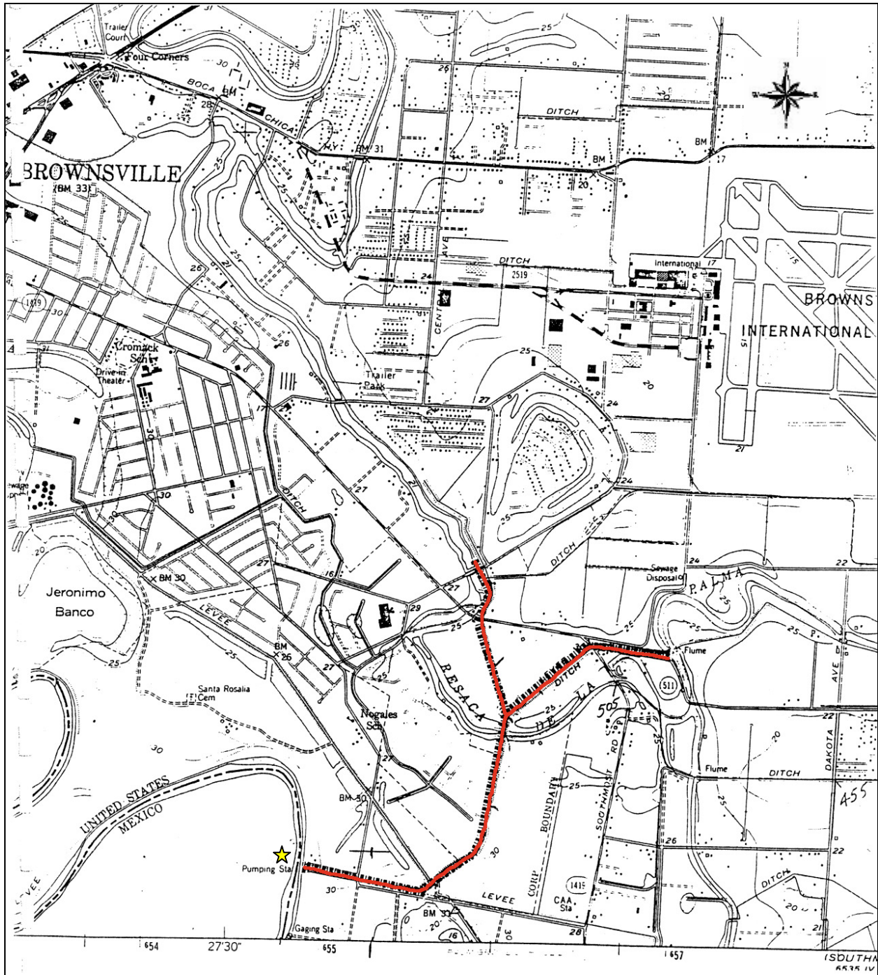
FIGURE 2. Partial Illustration of Brownsville Irrigation District, Highlighting the 2.5 Mile-Long Main Canal, 2001 (Holdar-Garcia & Associates).
