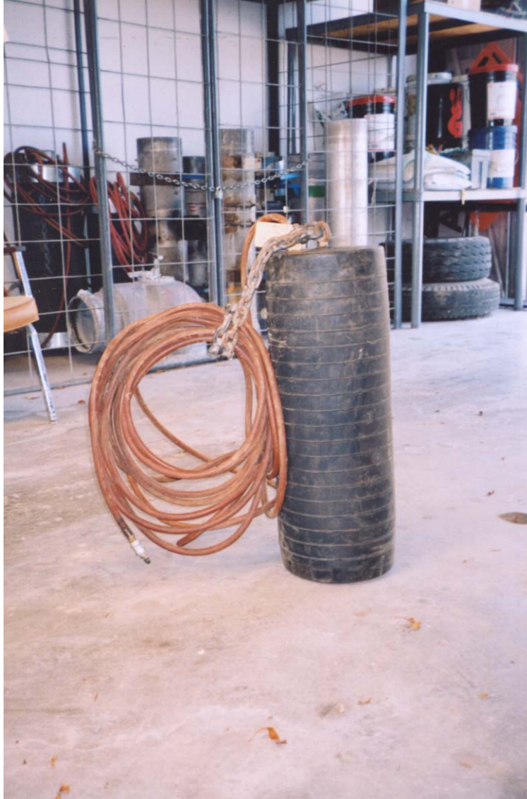
EXHIBIT C8. Pipe Balloon that is used to stop the flow of water within a pipe, usually for the purpose of maintenance, 2003.
