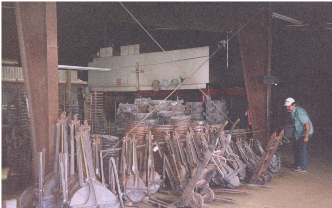
EXHIBIT C12. Completed Gates of Varying Size at HCID2 Machine Shop, 2003 (Stubbs).
