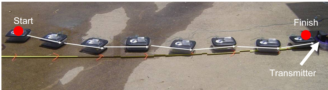
Fig. 4.2: First test of goal-seeking algorithm, 240 cm away, 30 cm off-center, 8 total iterations
