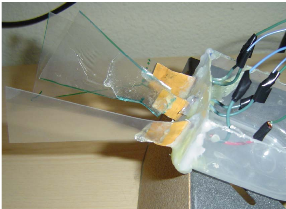
Fig. 2.16: Fins attached to IPMC strips with epoxy resin
