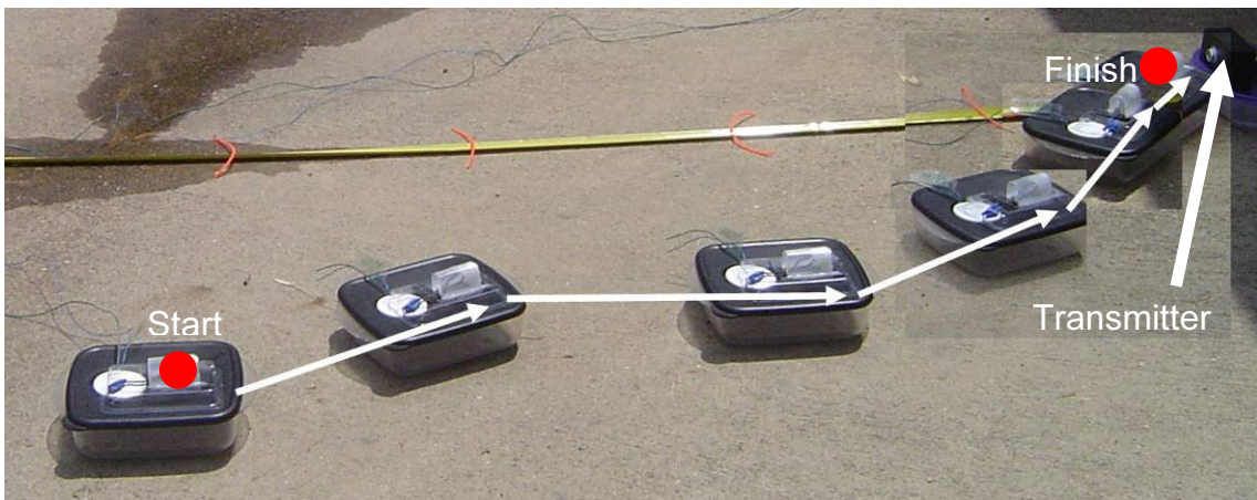
Fig. 4.3: Second test of goal-seeking algorithm, 120 cm away, 60 cm off-center to the left, 6 total iterations
