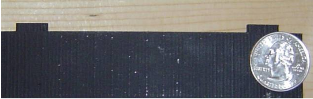
Fig. 2.4: Close up picture of vessel showing tabs to keep water shield in place
