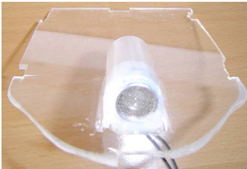
Fig. 2.17: Ultrasonic receiver encased atop the acrylic shield, sealed with silicone
