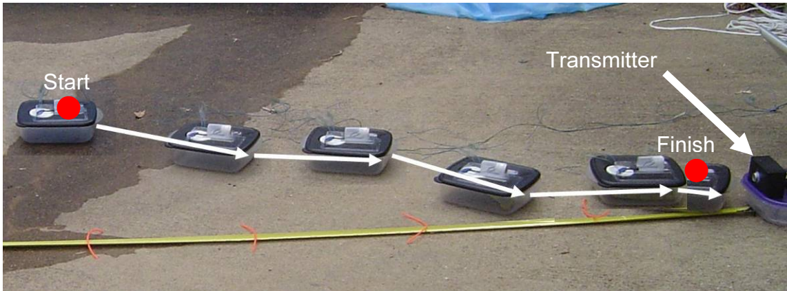
Fig. 4.4: Third test of goal-seeking algorithm, 120 cm away, 60 cm off-center to the right, 6 total iterations
