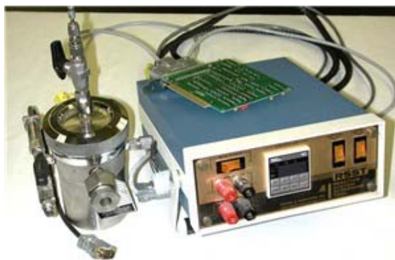
Fig.2.3. RSST including a pressure vessel and control unit ( http://www.chem.mtu.edu/~crowl/rsst.htm )
