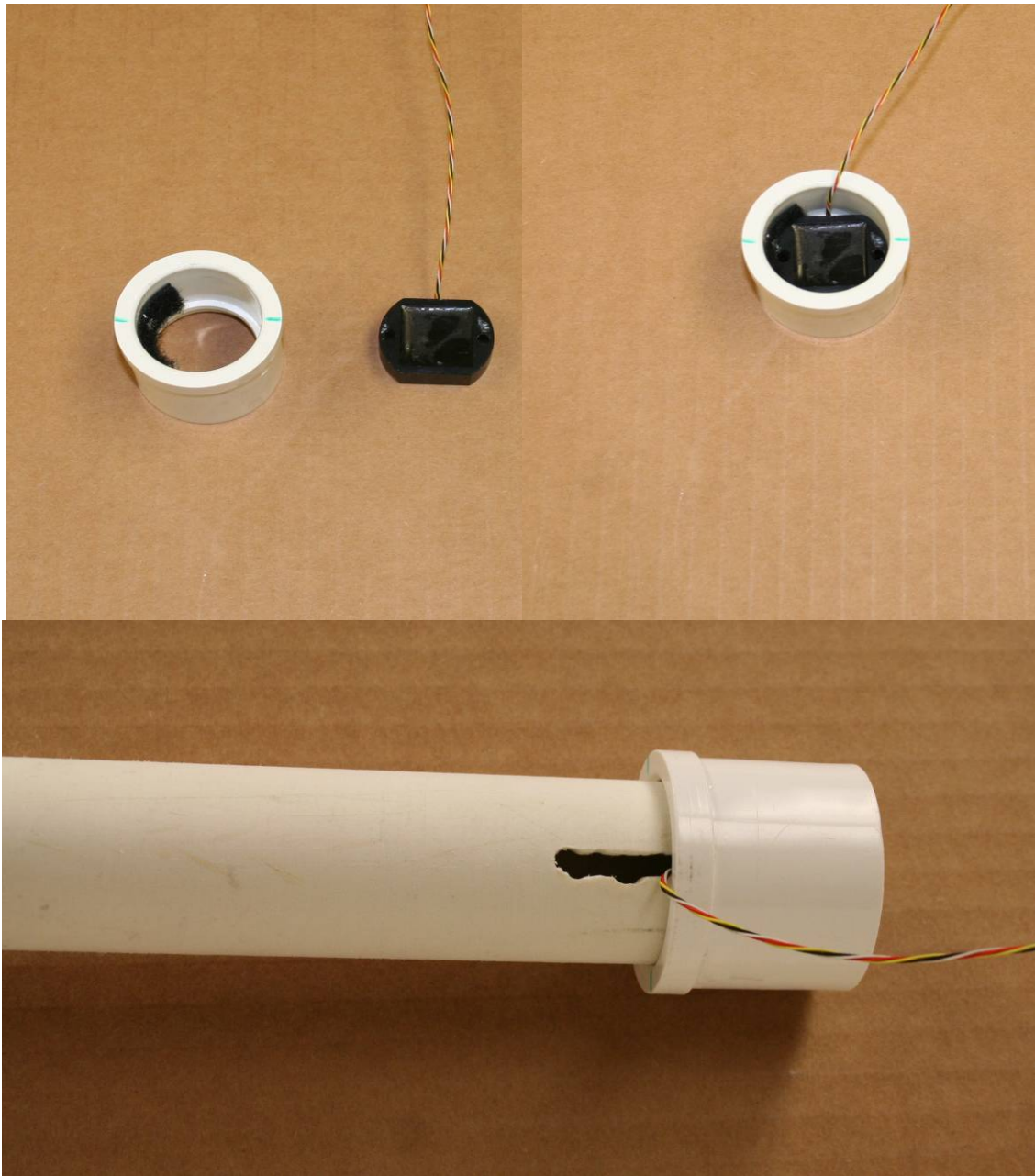
Figure 19. MEMS accelerometer installation. (Clockwise from upper left) MEMS accelerometer beside bushing, MEMS placed in bushing, 1 in. diameter pipe inserted in bushing used to place MEMS and bushing in receptacle.
