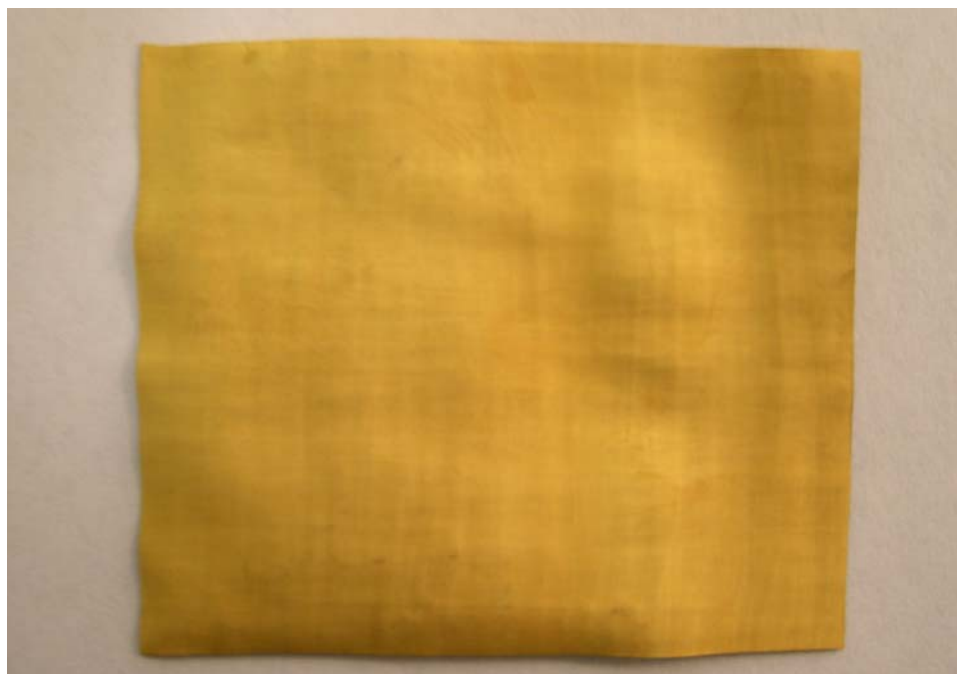
Fig. 2-2. Platinum- and gold-plated Nafion 117 membrane (Lithium counter ion).
