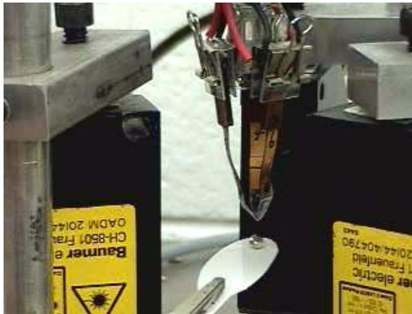
Fig. 6-14. First step of the pick-hold-drop operation.
