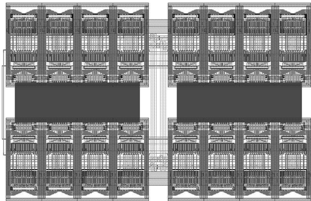
Fig. 59. Fourth level of hierarchy in the layout of the resonator. Each of these contributes 128 levels of the thermometer coding.
