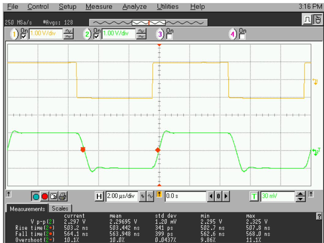
Fig. 92. 2.3 V_{pp} , 100 kHz unity gain step response.
