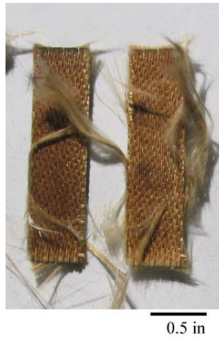
Figure 44. Aged Sample N-17 After Cutting for Mechanical Testing
