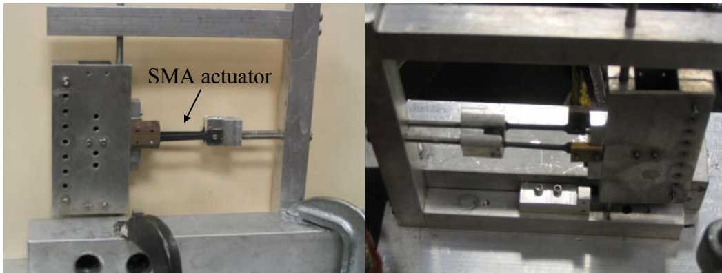
Figure 19: First Prototype SMA Actuation Setup
