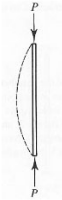
Fig. 10 Column under compressive loading with typical shape that may form as a result of buckling [15]
