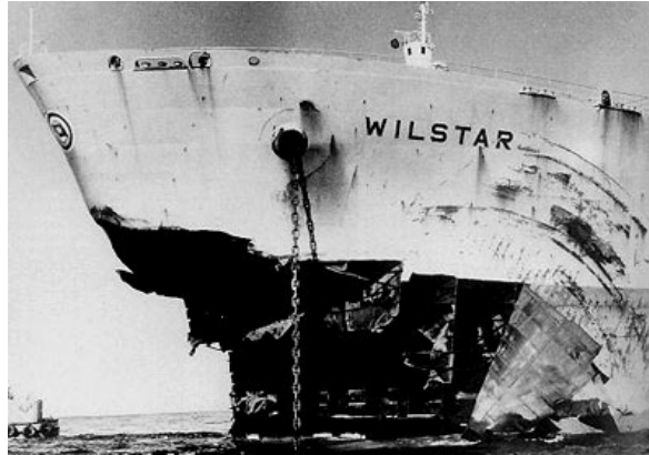
Fig. 1.2 Damage to the Norwegian tanker Wilstar , which was hit by a rogue wave in 1974.
