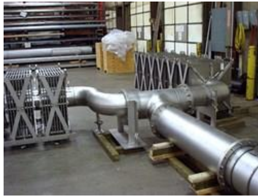
Figure 3-3. Example Sump Strainer [12]
