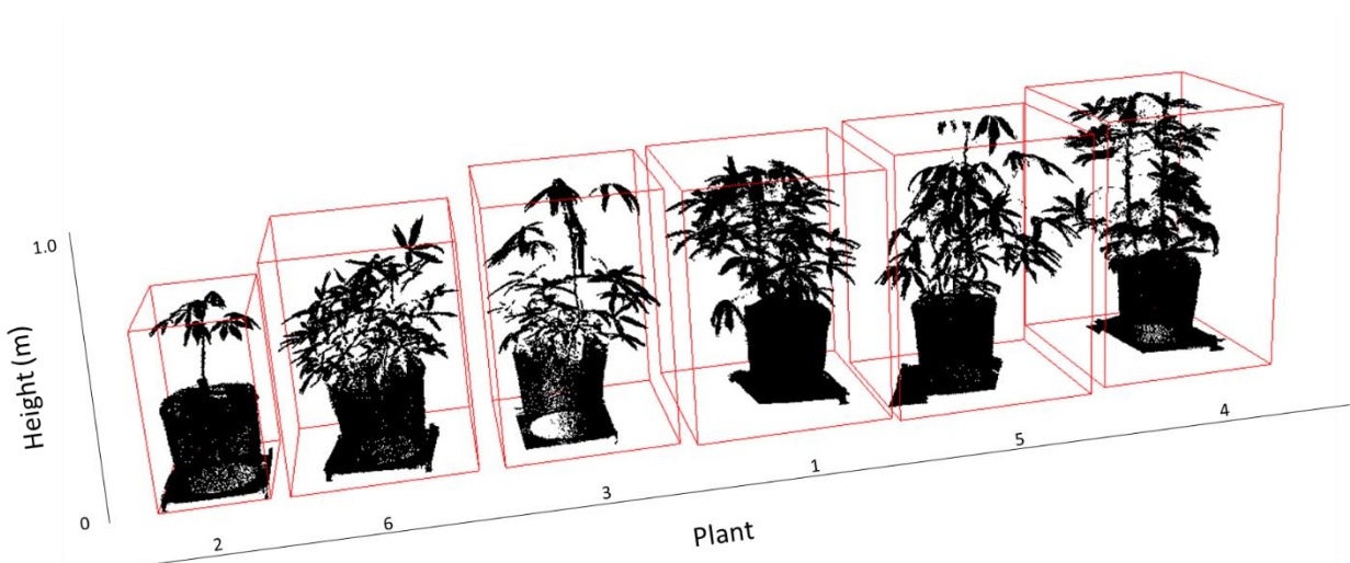
Figure 2. FARO models of the six cassava plants arranged by height, with the bounding box visible.
