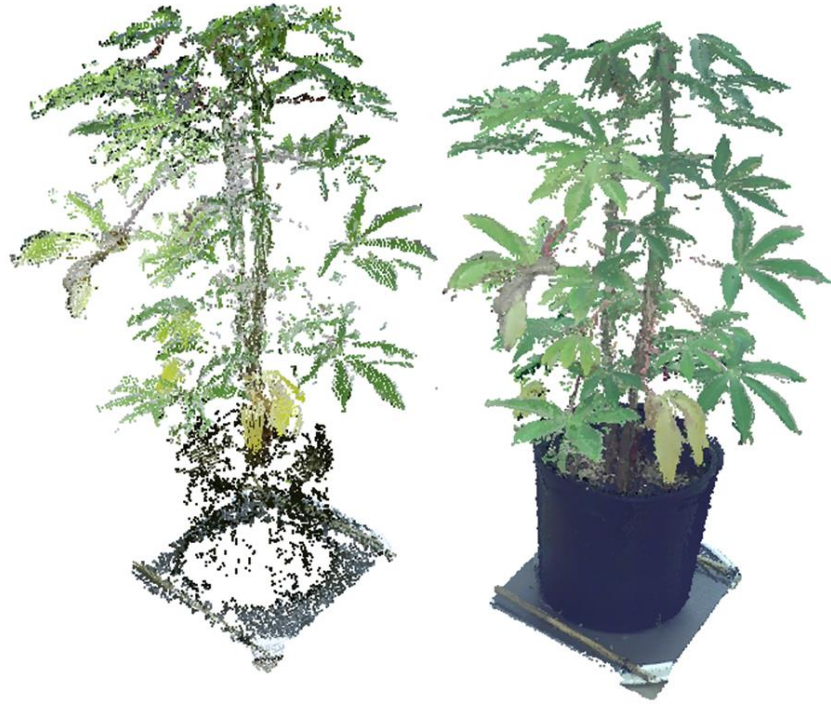
Figure 10. A side-by-side comparison of Plant 4 (Kinect on the left, FARO on the right). Note that the pot is lacking in point density for the Kinect model.
