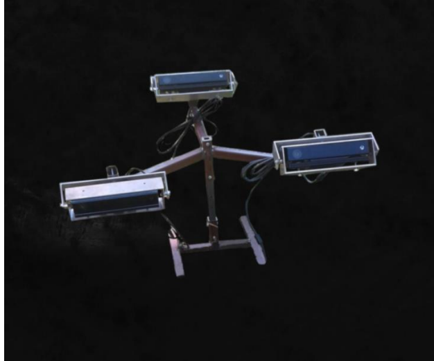
Figure 15. The Scorpion phenotyping platform utilizing three Kinect cameras to widen the field-of-view.
