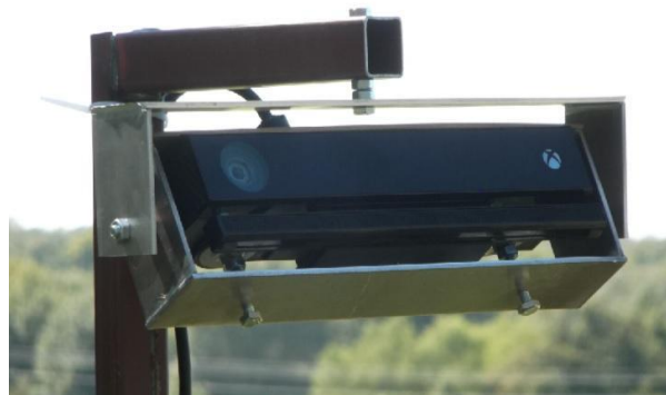
Figure 17. An adjustable Kinect sensor frame used to hold the camera in place with no movement.
