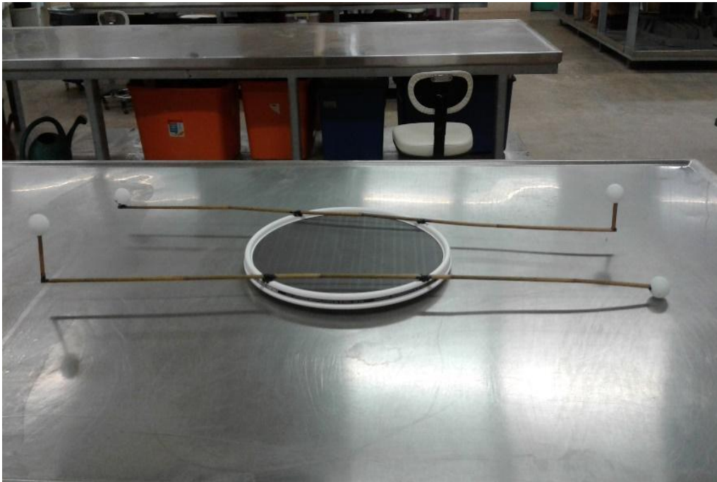
Figure 4. Modified turntable for plant rotation with table tennis ball targets for registration.
