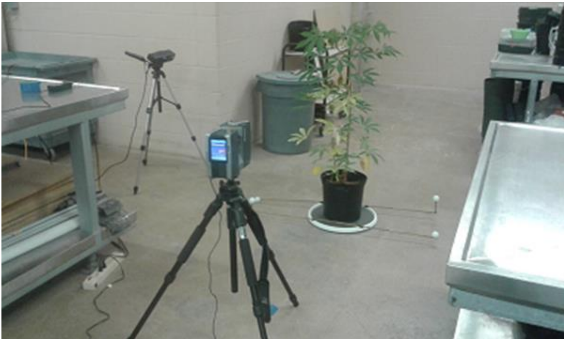
Figure 3. Simultaneous image capture process for the Microsoft Kinect V2 (left) and the FARO Focus 120 (right).
