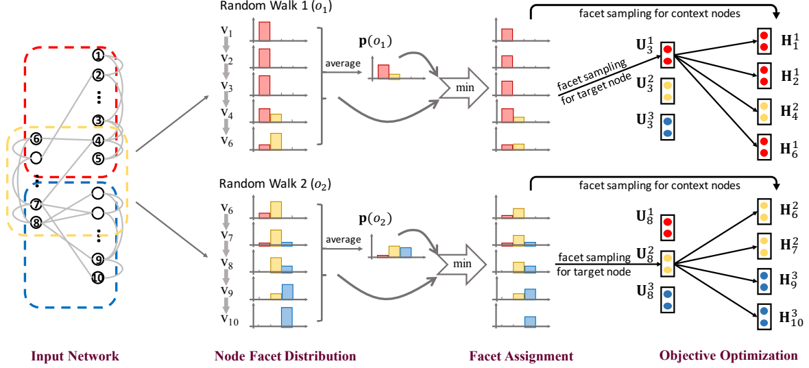
Figure 4.1: The overall training procedure of Polysemous Deepwalk. Each color refers to one facet (i.e., cluster in this case) in the input network. Each histogram visualizes a probability distribution. Note that the above network is only a toy example for illustration purposes, where numerical values do not reflect real results. Reprinted from [4].
