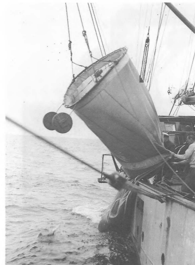
Figure 1.6 The “chariot,” a plankton net equipped with wheels for sampling just over the bottom, being taken aboard the research vessel Atlantis on a 1935 cruise. [O. E. Sette Collection, National Marine Fisheries Service]
