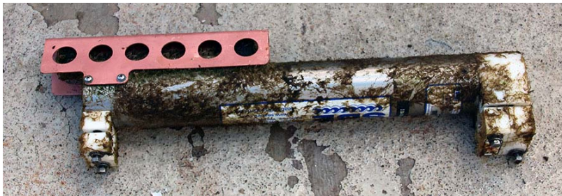
Figure A3-5. NTAS-18 SBE-37s from 10, 25, 40, 55 and 70 m (upper to lower).
