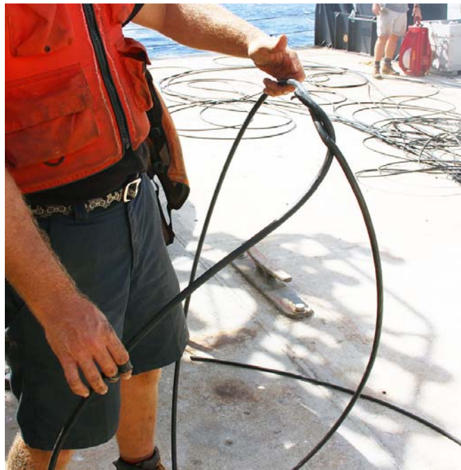
Figure 16. Lower end of the broken 500 m wire section from the NTAS-19 mooring. Permanent kinks indicated that the wire had looped back on itself.
