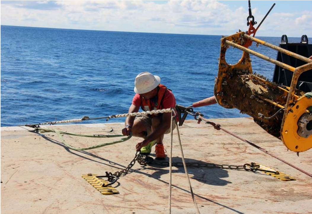
Figure 14. NTAS-18 drifting buoy recovery. The buoy has been recovered and the EM chain removed. Yale grips and Klein grips are used to take up tension on the wire below the bell mouth.
