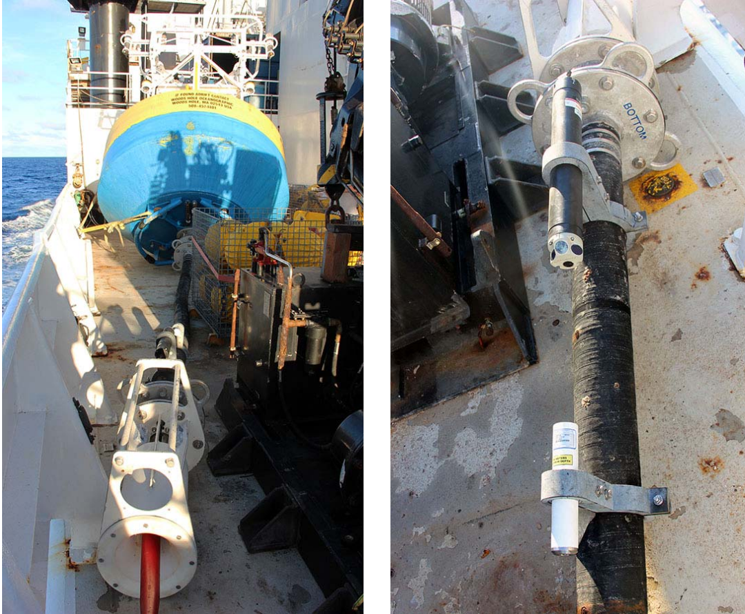
Figure 5. NTAS-19 buoy assembly on deck. (left) Wire termination, bell mouth, EM chain, universal joint and buoy base. (right) SBE-39 temperature sensor and Nortek current meter mounted on EM chain.
