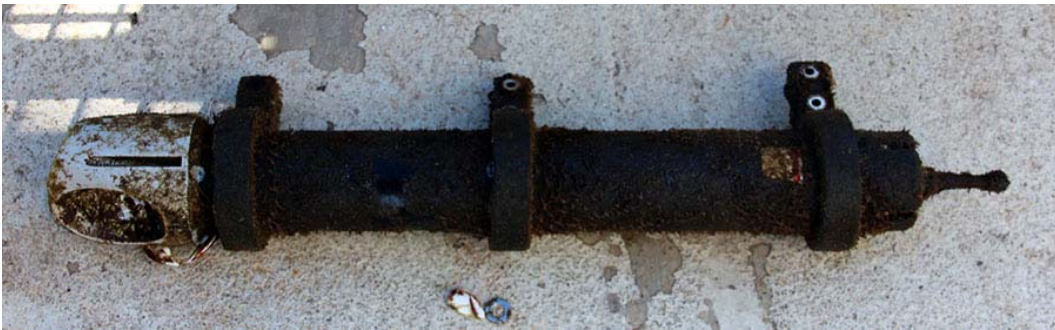
Figure A3-3. NTAS-18 Nortek current meter (13 m) and profiler (24 m).
