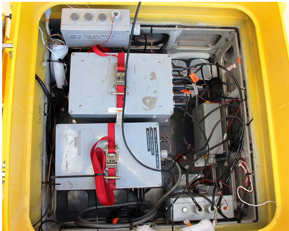
Figure 7. NTAS-19 buoy well showing major electronic components.
