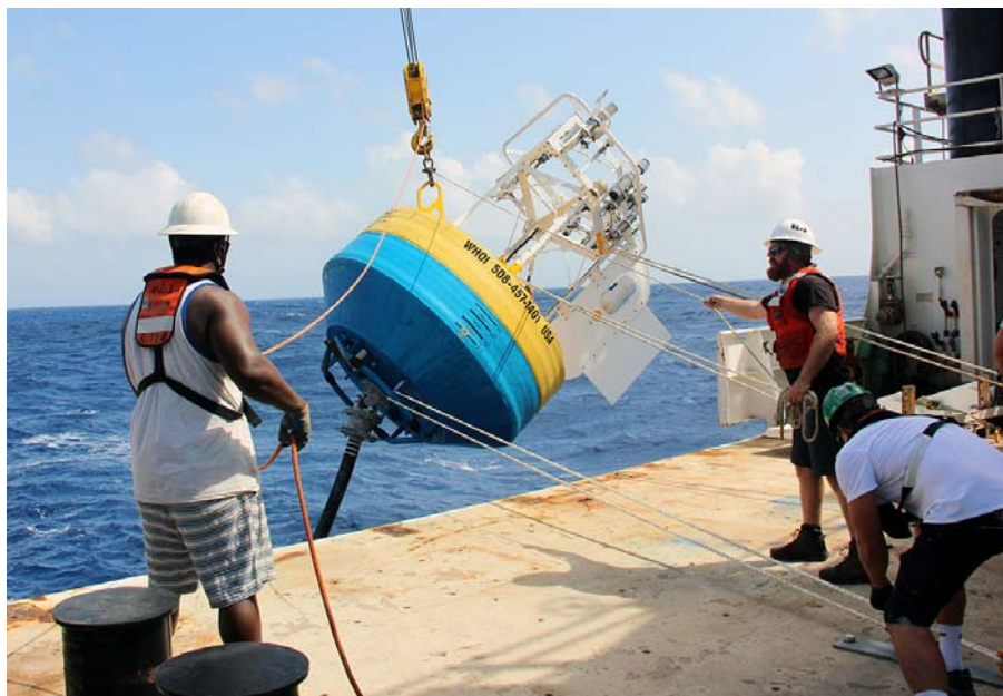
Figure 10. NTAS-19 buoy deployment. Tag lines for the crane headache ball, quick release, buoy base, buoy deck, and buoy tower can be seen.
