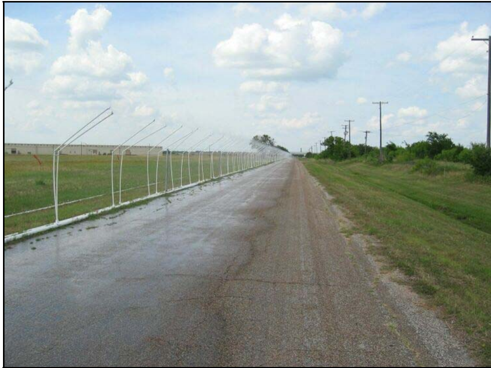
FIGURE 24 Rain Simulator Wetting the Road.
