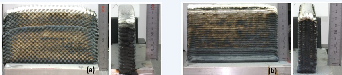
Figure 4: Physical quality of aluminium 2319 WAAM walls produced: (a) oscillated deposited wall; (b) parallel deposited
