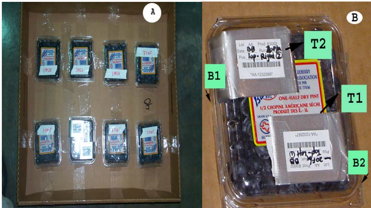
Figure 3-3. Experimental setup for irradiation of blueberry fruit. (A) placement of fruit on the trays, (B) location of film dosimeters on the product.
