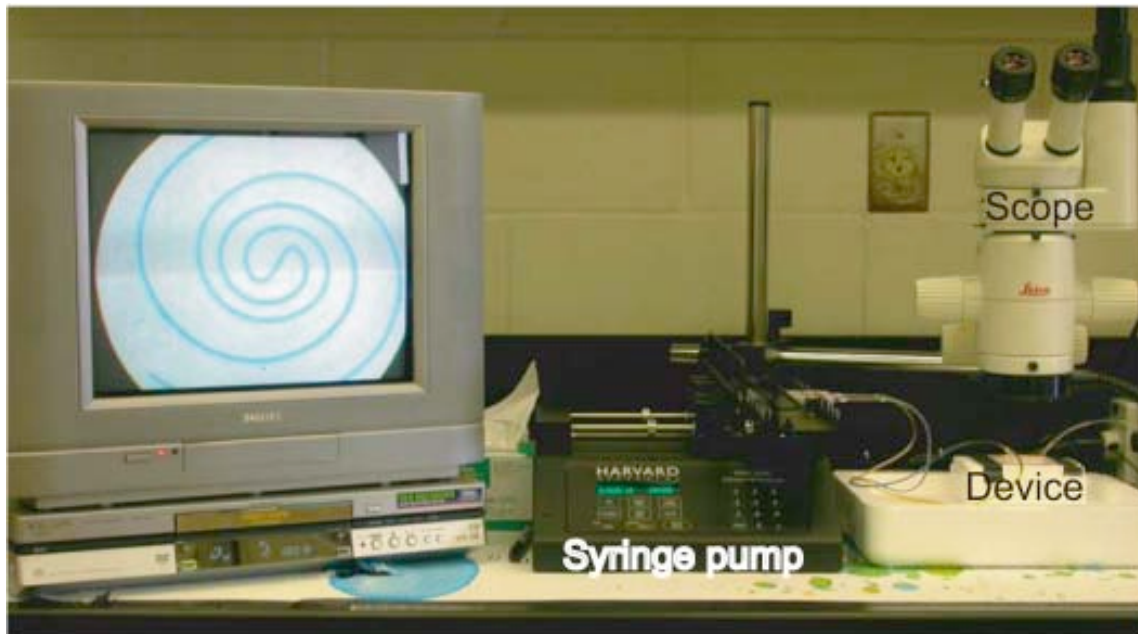
Figure II-15. Top-view imaging setup.
