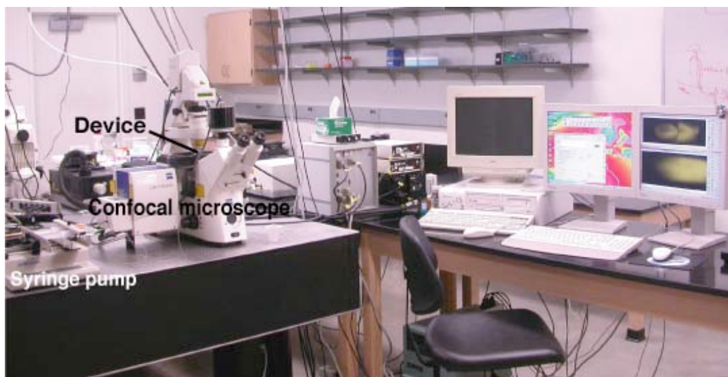
Figure II-17. Cross-sectional imaging using a LSM 5 PASCAL confocal microscope.
