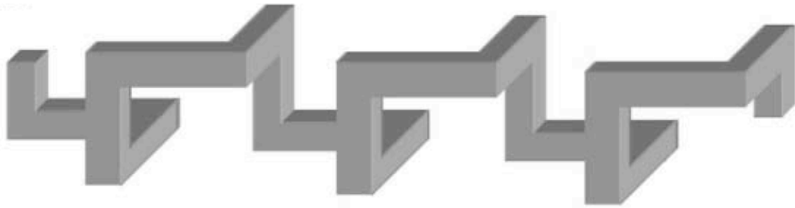
Figure I-19. Three-dimensional stirrer comprised of a series of square bends. Reprinted from International Journal of Heat and Fluid Flow , 24, Yi, M.; Bau, H. H. The kinematics of bend-induced mixing in micro-conduits, 645-656. © 2003, with permission from Elsevier.
