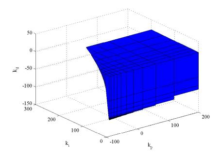
Fig. 6.: Set of PID Controllers Satisfying SPR Condition 2
