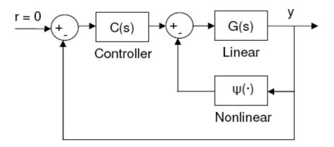
Fig. 5.: Control Structure of One-Link Robot with a Flexible Joint
