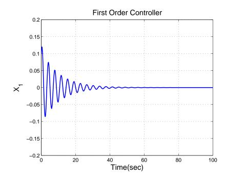
**Fig. 14.:** Response of the Robot's Angular Position with a First Order Controller  $(k_1^* = -20, k_2 = -50, k_3 = 1)$
