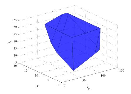
Fig. 7.: Set of PID Controllers Satisfying SPR Condition 3
