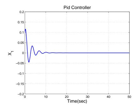
**Fig. 9.:** Response of the Robot's Angular Position with a PID Controller ( $k_p = 50, k_i = 5, k_d = 15$ )
