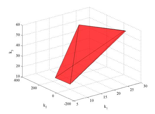
Fig. 19.: Set of Stabilizing First Order Controllers.
