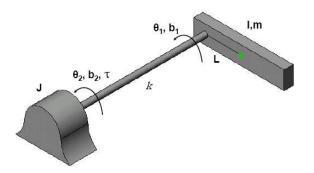
Fig. 4.: One-Link Robot with a Flexible Joint
