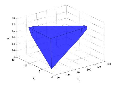
Fig. 8.: Set of Absolutely Stabilizing PID Controllers
