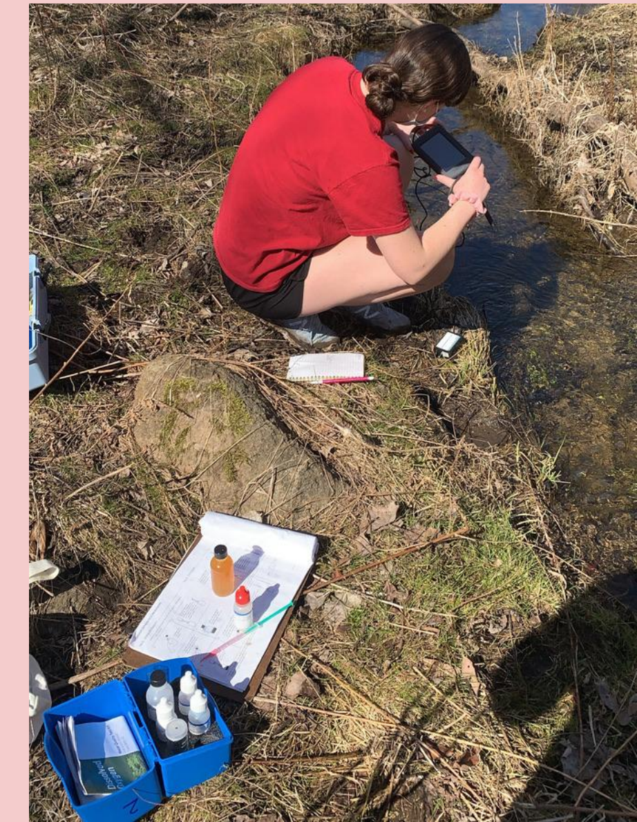
Fig. 2. Recording the temperature of the water and dissolved oxygen content at location three, Wilkins Creek.
