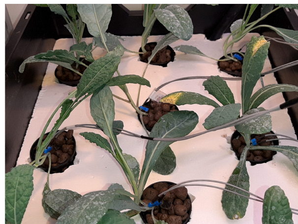
Fig. 4. The black kale plants under study equipped with the wired connection of the electrodes.
