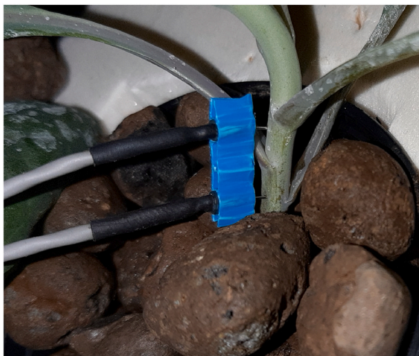
Fig. 3. Detail view of the inserted electrodes into the plant's stem.
