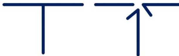
Fig. 24. The new deposition strategy proposed by the Authors for T-Crossings. The original curves from the "First Layer Curve List" (left) and the toolpath optimized for the T Crossing (right).
