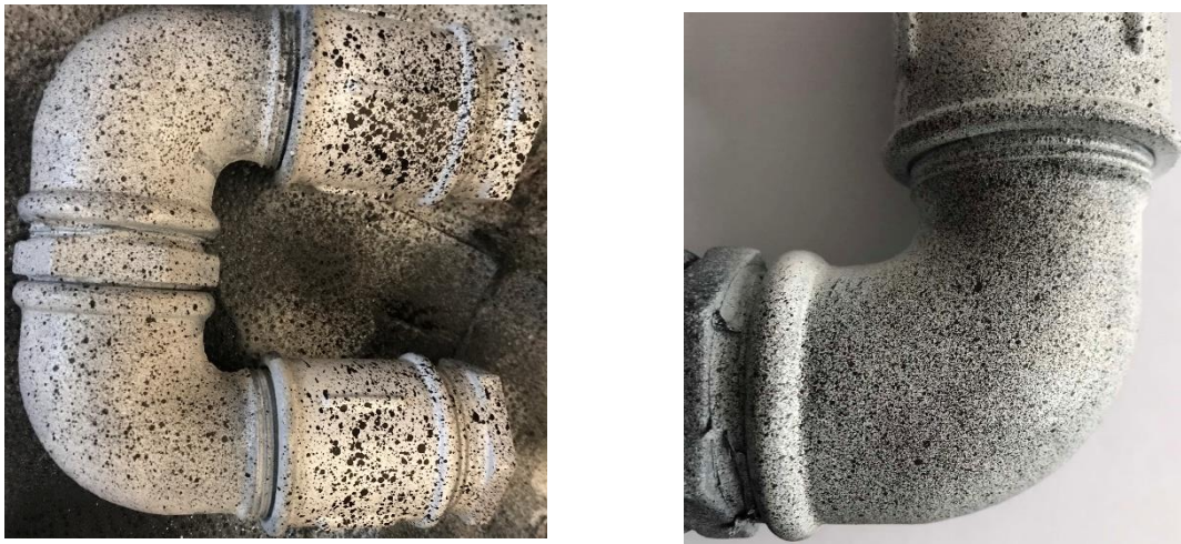
Figure 8. The surface preparation of the U pipe rough spray (left) and the fine spray (right)
