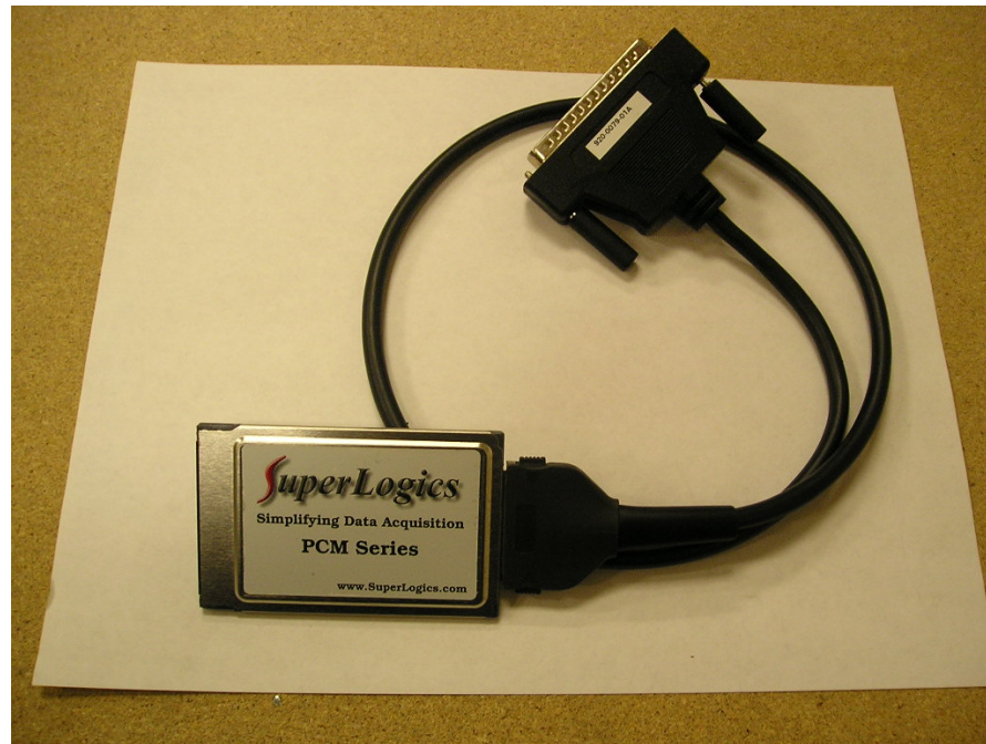
Figure 4.1. The PCMDIO card with the CP-1037 adapter cable
