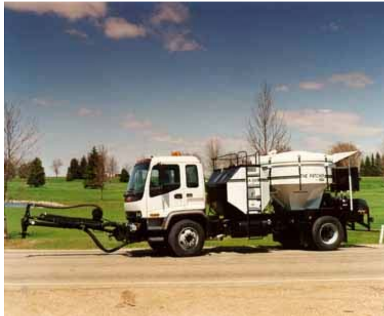
Figure 1.3. Spray injection device – self-contained unit (Source: www.tfhrcc.gov/focus/archives/focus399/0399cal.htm )
