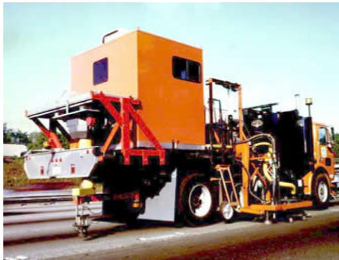
Figure 2.1. The ACSM developed by the AHMCT at UC Davis (Source: www.ahmct.ucdavis.edu )
