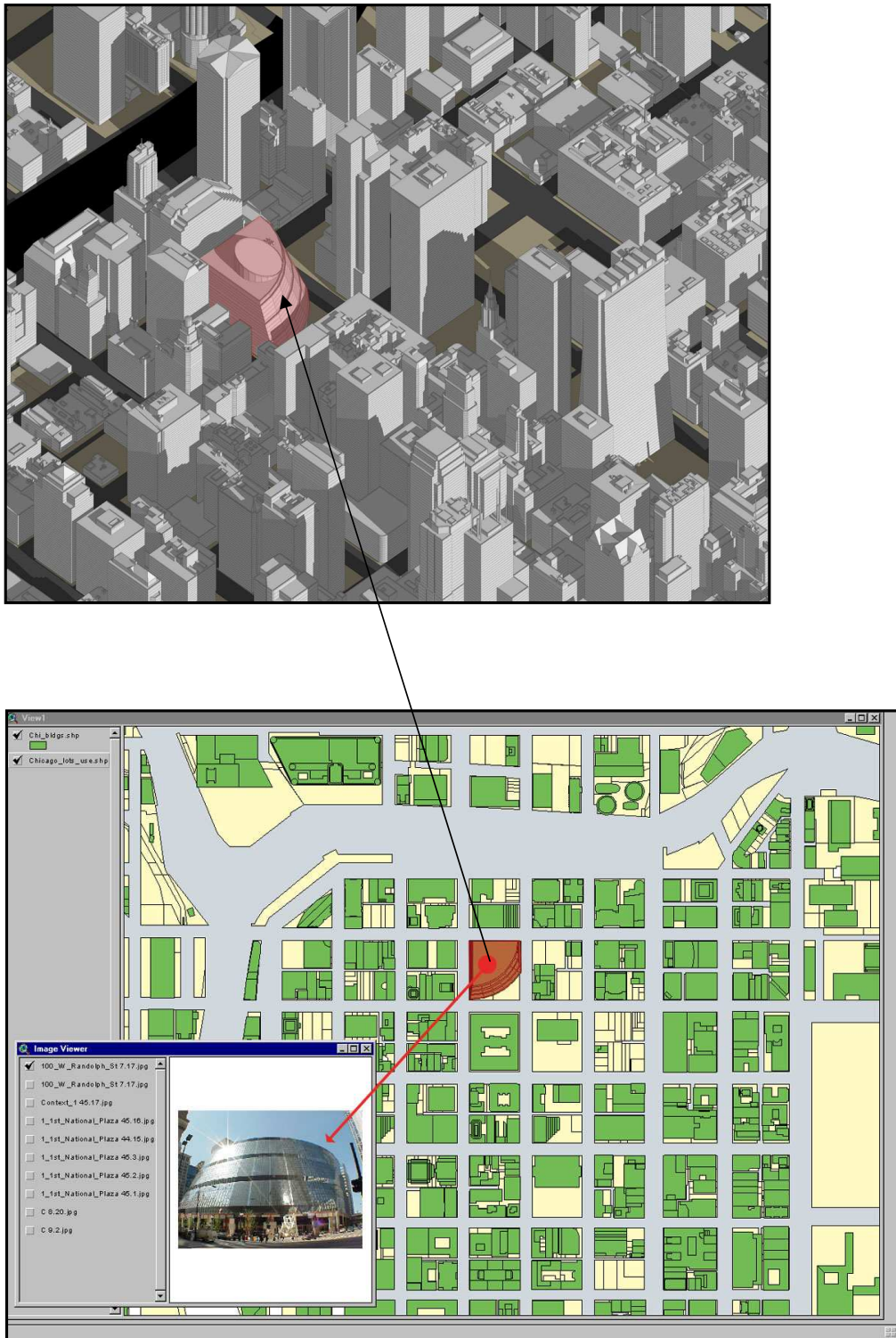
Figure 4.4. Integrating multiple types of spatial data and representing it with various levels of representation (EarthData Solutions 2005).
