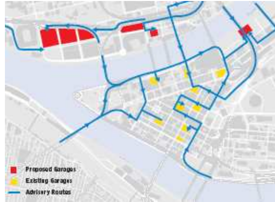
Parking Advisory System: Shown are some of the proposed routes that could be equipped with electronic signs.
