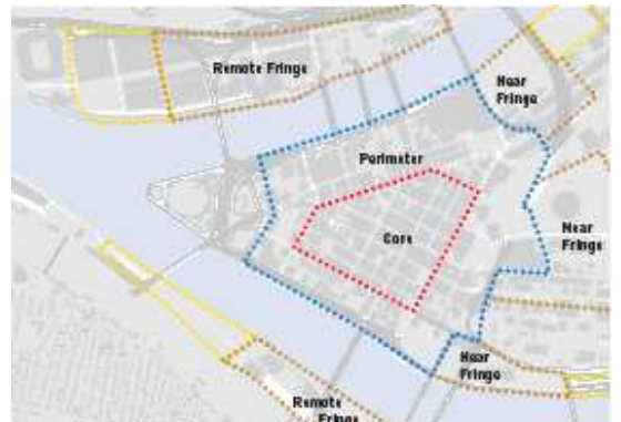
Shared Parking Options: The development strategy involved adding from 3,000 – 5,000 spaces in demand. To address this problem, a five-tiered system has been proposed. The zones, characterized by distinct levels of convenience, rate structures and a distinct market, would include core, perimeter, near fringe, remote fringe and satellite.
