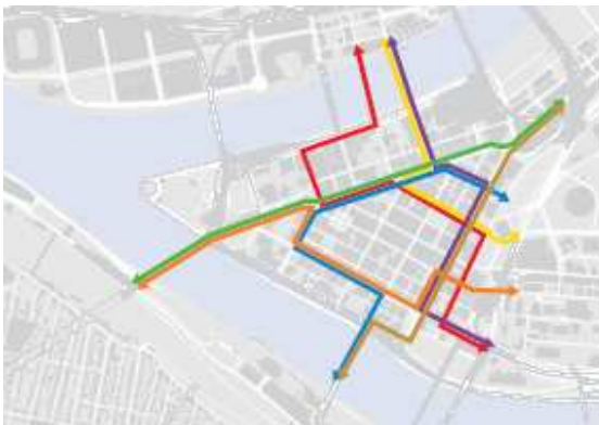
Through Bus Routing Concept: The concept brings buses in one corridor and out another which is shown in the schematic of a through routing system with each corridor color coded as it comes in and out of downtown.
