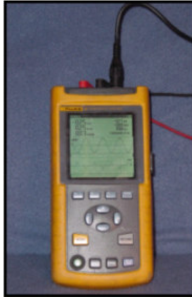
Fig. 38. Fluke 43 Power Quality Analyzer
