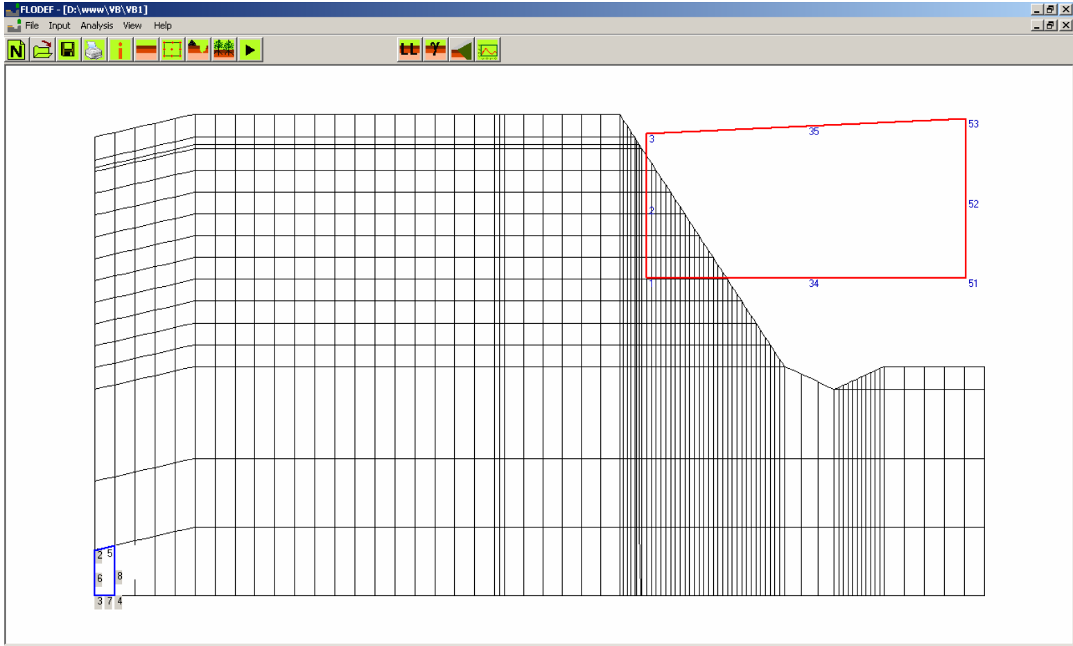
Figure 3.23 FEM mesh generated in the program
