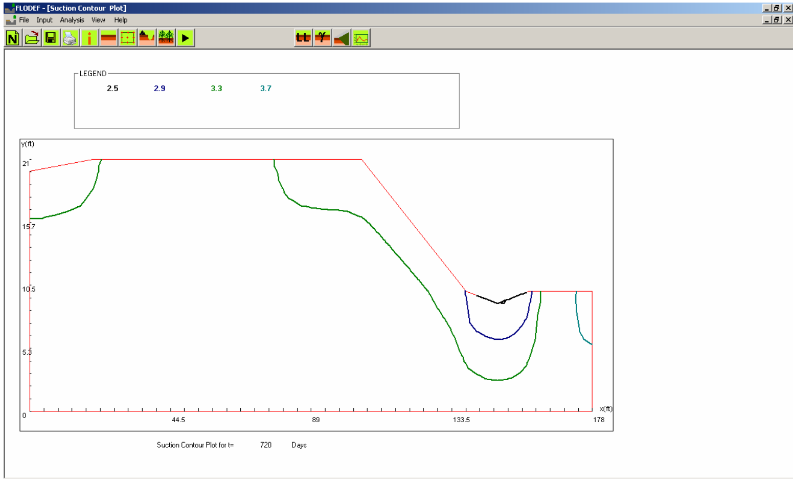
Figure 3.16 Output plot 4: contour plot (suction)
