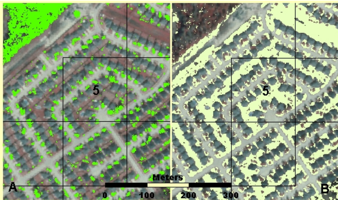
Figure 4.16. A typical newly developed residential neighborhood. Vegetation measurement grids overlay the 1995 false color near-infrared composite DOQQ. The mean at-satellite surface temperature for sample area #5 is 301.049 Kelvin. (A) The green areas represent Total Tree Canopy: 9.79% for sample area #5. (B) The light green areas represent Low-Level Vegetation: 36.19% for sample area #5.
