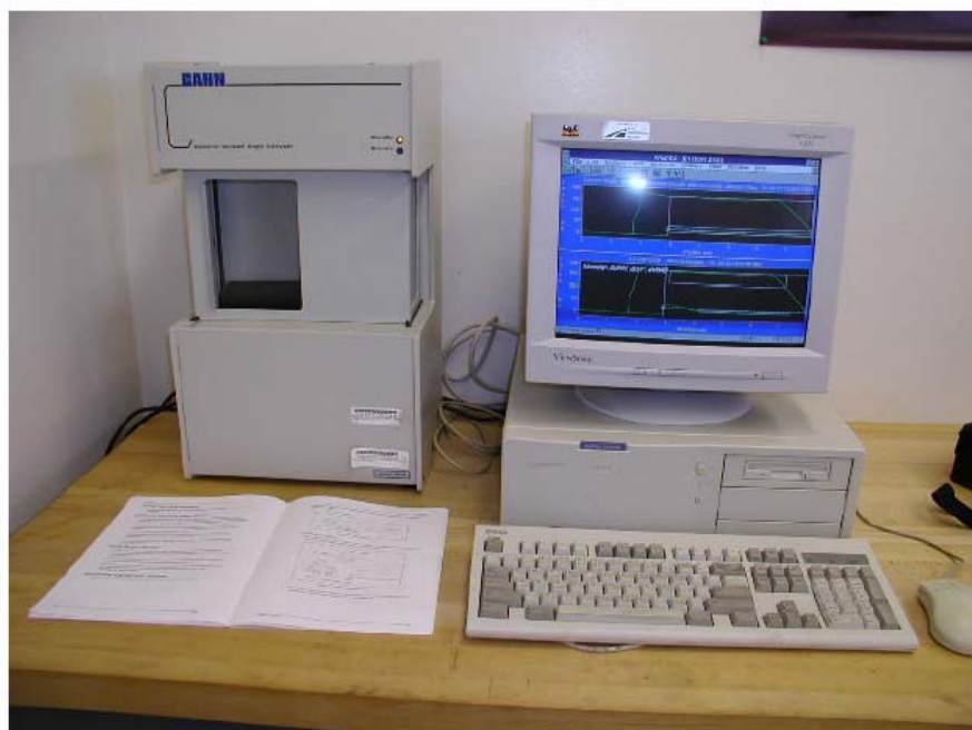
Fig. 5-11. The DCA Force Balance and Computer Setup - Wilhelmy Plate Test
